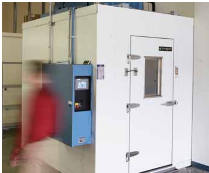
The UPS temperature-humidity chamber helps identify the proper packaging for your sensitive shipments.
